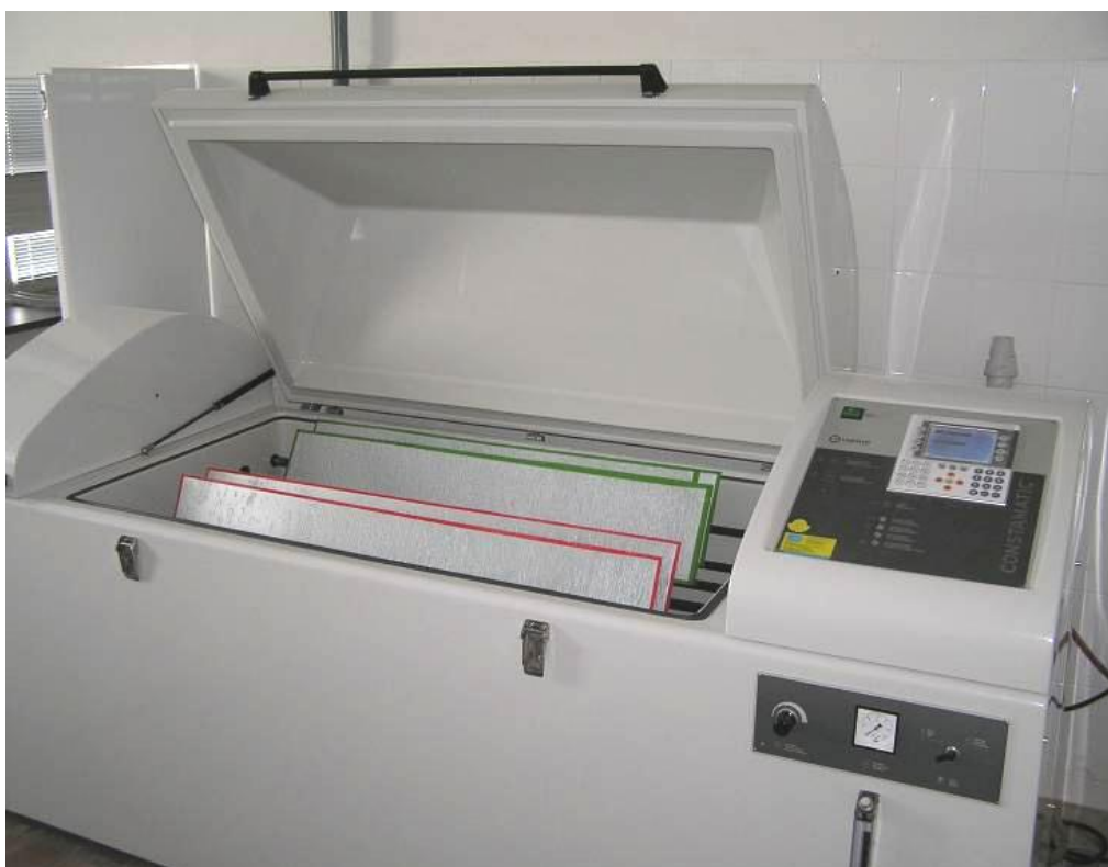
Fig. 2 Corrosion chamber SKBWF-1000A TR
