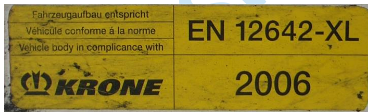
Vehicle body marking according to EN 12642
