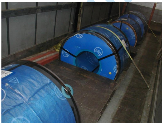
Not proper use of coil-well covers between neighbouring coils – covers can tilt up during coil movement
