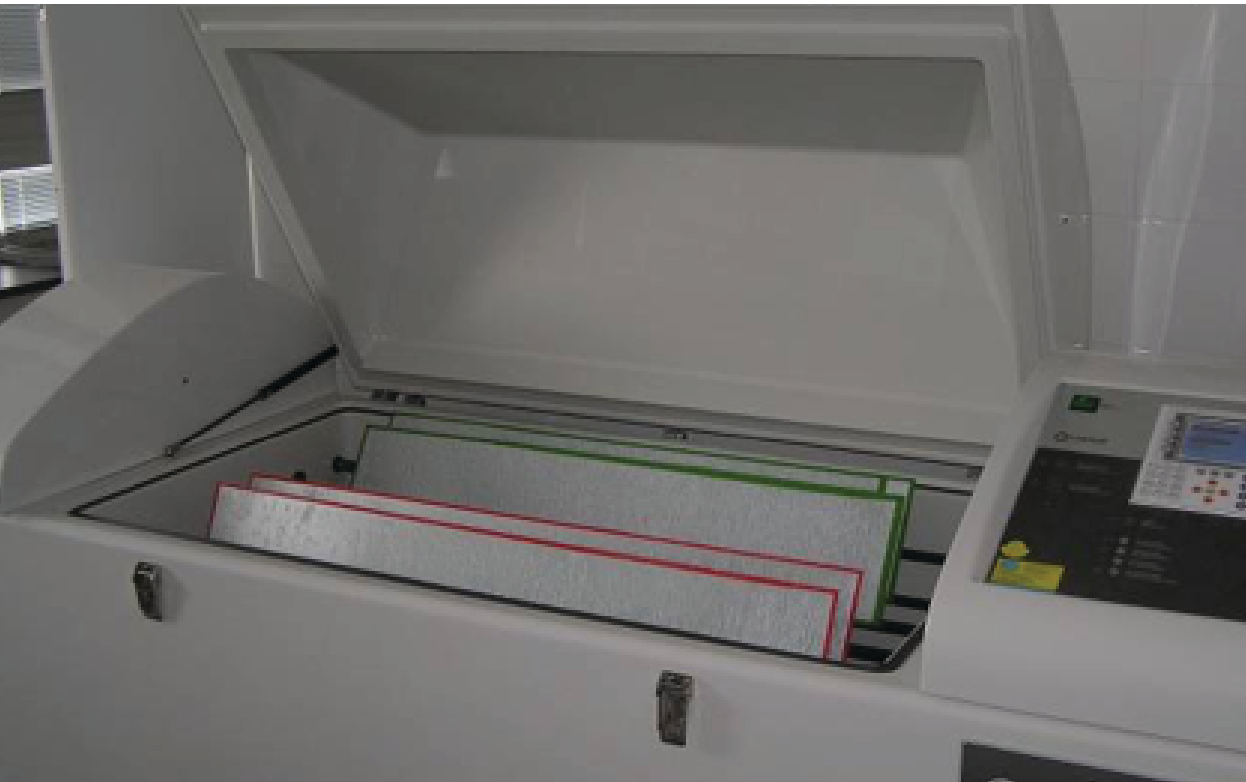
Figure 2 Chamber used for corrosion tests
